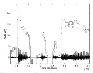
Figure 6: Comparison between FDD (dashed) and CDD approach (solid) in terms of SNR per frame versus time with  $\alpha = 0.98$ , P=3, 1 iteration and input SNR of 15 dB.
