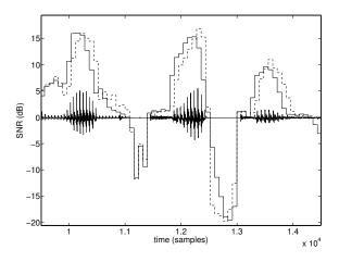
Figure 2: Comparison of FDD approach (dashed) versus BDD approach (solid) in terms of SNR with  $\alpha = 0.98$ .
