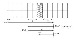
Figure 4: *Procedure for iterative combined forward-backward decision directed approach.*
