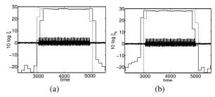
Figure 1: Noisy speech signal with  $\xi$  estimated by (a) FDD approach (b) BDD approach (solid) and the true SNR (dashed).
