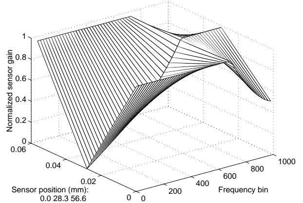
**Fig. 3.** Normalized sensor gain with PCA-based subspace selection
