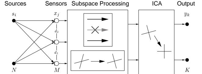
**Fig. 1.** General framework of overdetermined BSS
