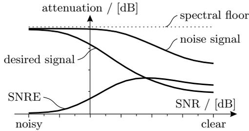
Figure 8: Suppression capability in respect to the input SNR
