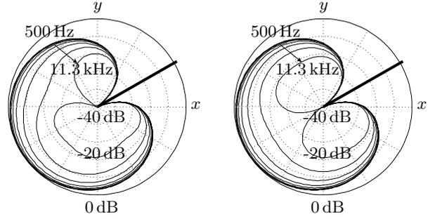
Figure 6: Polar Pattern of Array 1 and 2 for  $\varphi_0 = 30^\circ$
