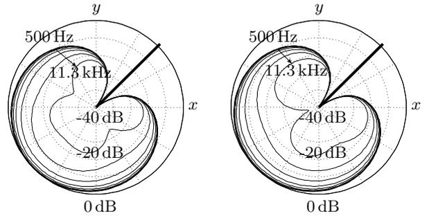
Figure 7: Polar Pattern of Array 1 and 2 for  $\varphi_0 = 45^\circ$
