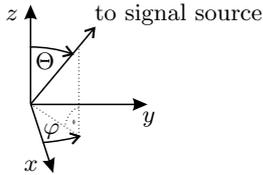
Figure 4: Definition of the angles  $\varphi$  and  $\Theta$
