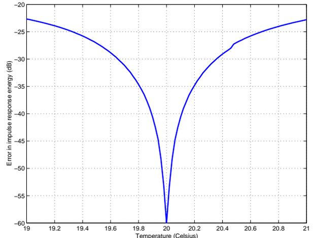
**Fig. 2.** Predicted misalignment error as a function of temperature for 10 cm microphone to loudspeaker spacing.
