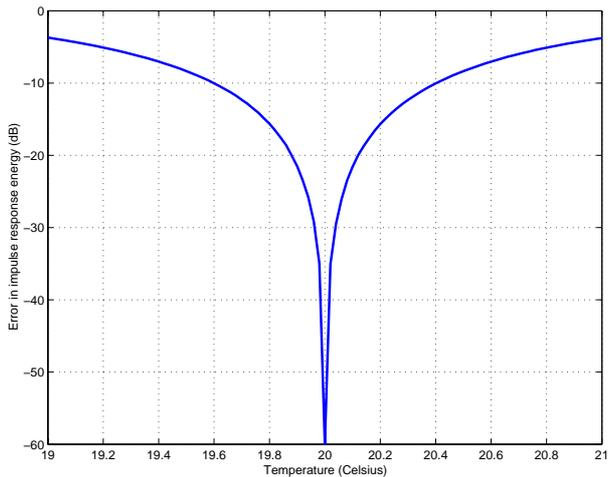
**Fig. 3.** Predicted misalignment error as a function of temperature for 2 m microphone to loudspeaker spacing.
