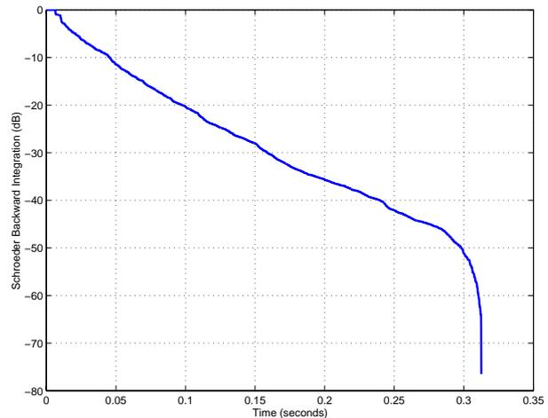
**Fig. 4.** Schroeder backward integrated room impulse response with 2 m spacing between the microphone and loudspeaker.
