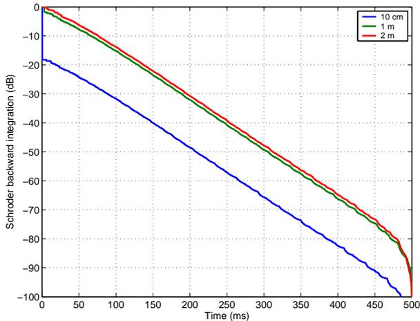
**Fig. 1.** Image model room impulse response with 10 cm, 1 m, and 2 m spacing between the microphone and loudspeaker.
