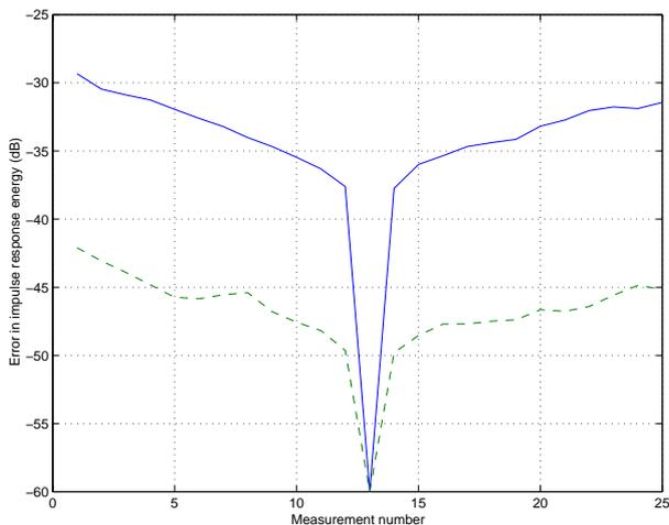
**Fig. 5.** Measured sequential variation in the room impulse response for 10 cm (dash) and 2 m (solid) microphone-loudspeaker spacings. The reference measurement is the center measurement.
