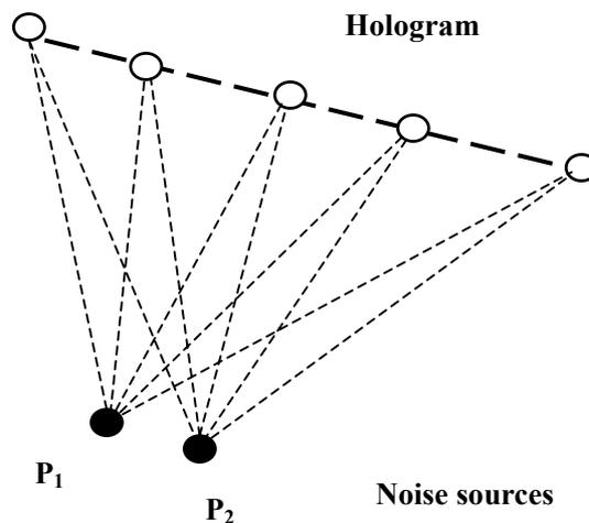
Fig. 2 One dimensional model of two noise sources.
