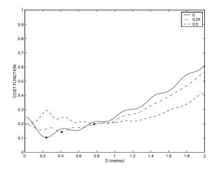
Figure 1: Variation of output noise power (12) versus intersensor spacing D, for three different positions of the source signal ( $x_s = 0, 0.25, 0.5$  m).
