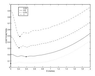
Figure 2: Variation of (16) versus intersensor spacing D at a frequency of 1000 Hz for a two-element array, with four different source distances ( $y_s = 0.25, 0.5, 0.75, 1$  m).
