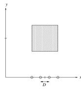
Figure 4: Geometry for broadband example. Source locations are indicated by the shaded region, microphone location are denoted by the circles.
