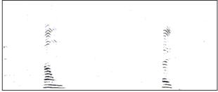
Figure 6. Power Spectrum of the Speech Trace after Spectral Subtraction
