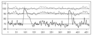
**Figure 7.** Instantaneous energy of the Noisy Speech Trace from Figure 4 (upper trace), of the Joint Process Estimation Error from Figure 5 (middle trace), and of the Speech Trace after Spectral Subtraction from Figure 6 (lower trace).
