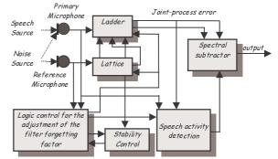
**Figure 1.** General framework of the proposed methodology: A Lattice-Ladder Filter is combined with a Spectral Subtractor.
