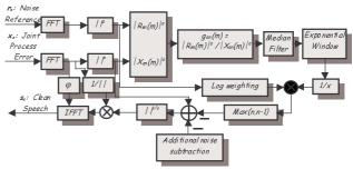
Figure 3 Specific Spectral Subtraction method being proposed
