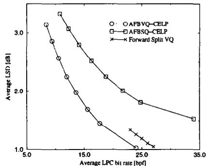
Figure 3: Comparison of AFBSQ, AFBVQ, and split VQ [5] in terms of LSD.
