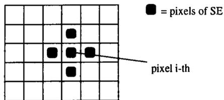
Fig. 1: Example of  $B_i$  centred on  $i$ -th pixel
