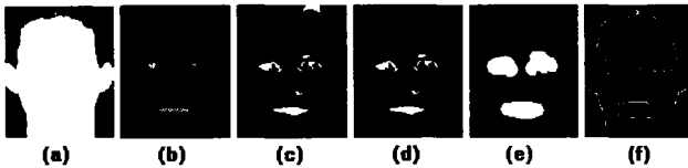
Fig.4. Steps of proposed processing method: face area (a), top-hat (b), binarized top-hat (c), part of binarized top-hat included in face area (d), feature areas (e), feature areas + contour of face area (f).
