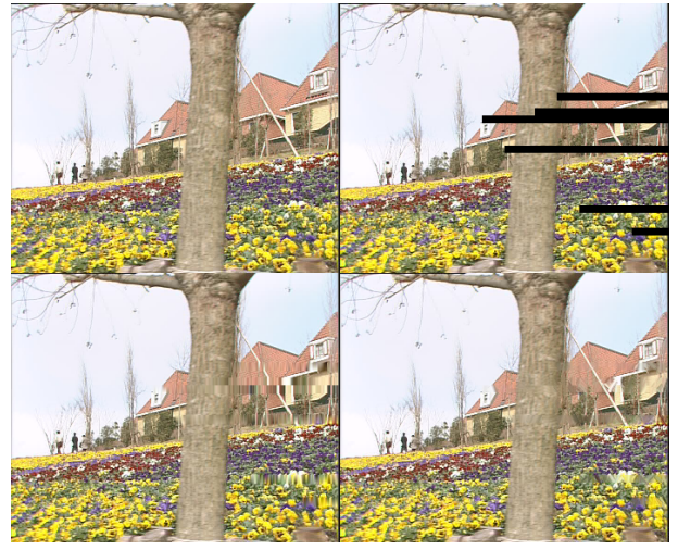
Figure 4: Frame 0: Error Free, PSNR = 32.2193 (top-left), Erroneous, PSNR = 15.7172 (top-right), processed by method [1], PSNR = 26.1087 , (bottom-left) and by Spatial S/M EC method (using anisotropic diffusion), PSNR = 26.4613 (bottom-right).
