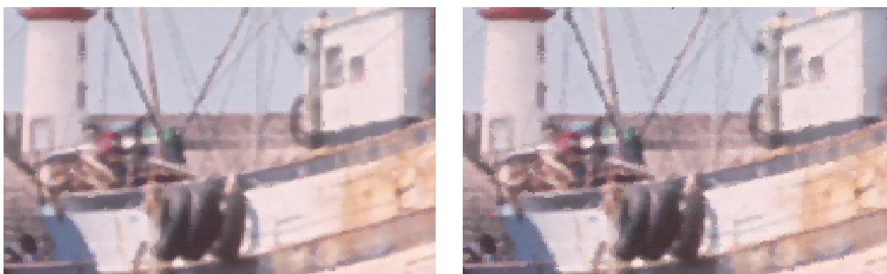
Figure 10: Y-U-V noisy image, filtered by a 3 \times 3 mm filter (left) and by a 3 \times 3 VML_2 filter (right).
