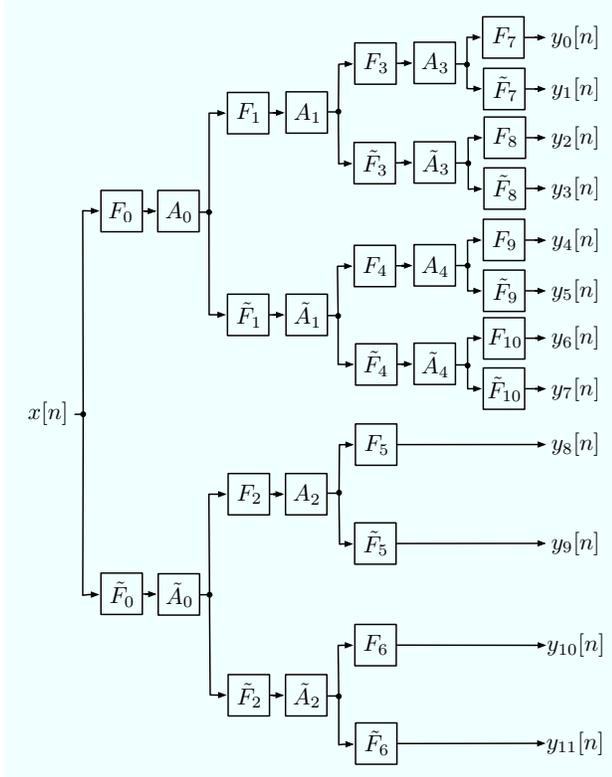
Fig. 3. Example 12-band complementary IIR filterbank.
