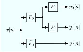
Fig. 2. Example of a 3-band complementary IIR filterbank implemented using a cascade of two 2-band complementary IIR filters.
