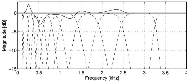
Fig. 5. Magnitude frequency responses of the 12 bands (dashed) and magnitude frequency response of the sum of the 12 bands with (bold solid) and without (thin solid) all-pass filters.
