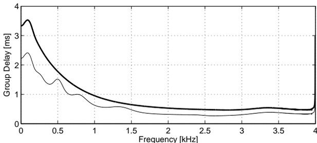
Fig. 6. The group delay of the impulse response of the sum of the bands with (solid) and without (thin) all-pass filters.
