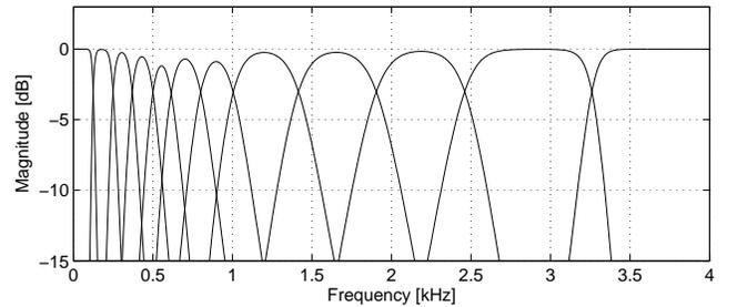
Fig. 4. Magnitude frequency responses of the 12-band example filterbank.
