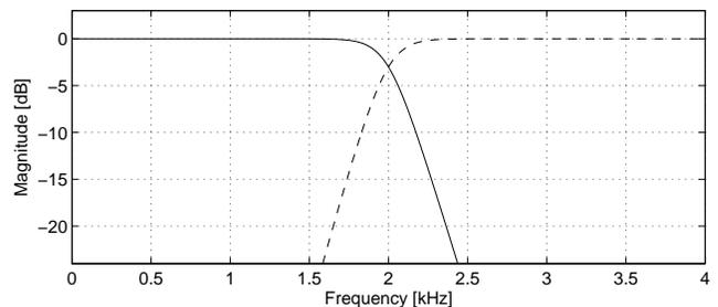
Fig. 1. The magnitude response of a low-pass filter (solid) and its complementary filter (dashed).
