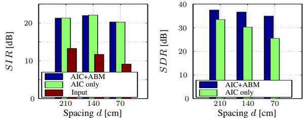
Fig. 6. SIR and SDR values calculated at the inputs (averaged over all channels) or after convergence of the residual cross-talk canceler (both with or without ABM), in the three-channel case.
