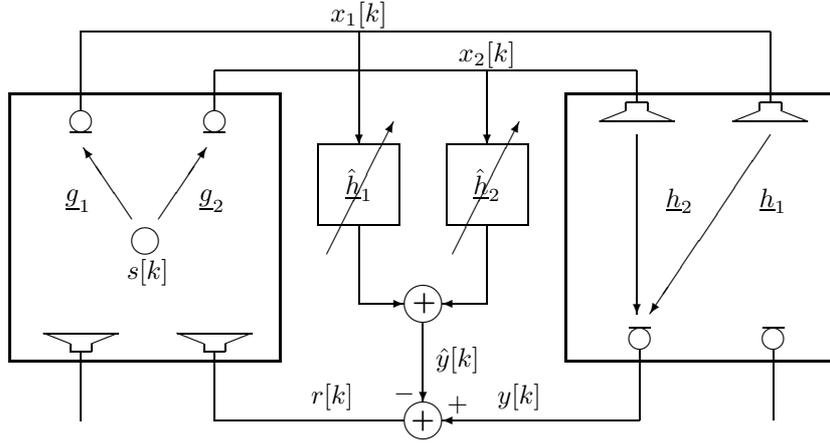
Figure 1: Schematic diagram for SAEC.
