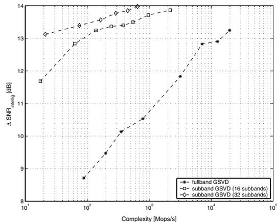
Figure 3: Improvement in  $\text{SNR}_{\text{intellig}}$  of fullband and subband GSVD as a function of complexity (Mops/s) for  $M = 4$ ,  $d_f = d_g = 1$ .
