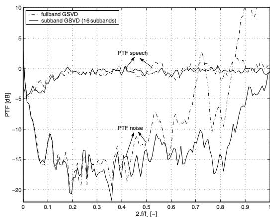
Figure 4: Power Transfer Function of speech and noise signal obtained with fullband and 16 subband GSVD for  $M = 4$  and a temporal window  $LD = 24$ .
