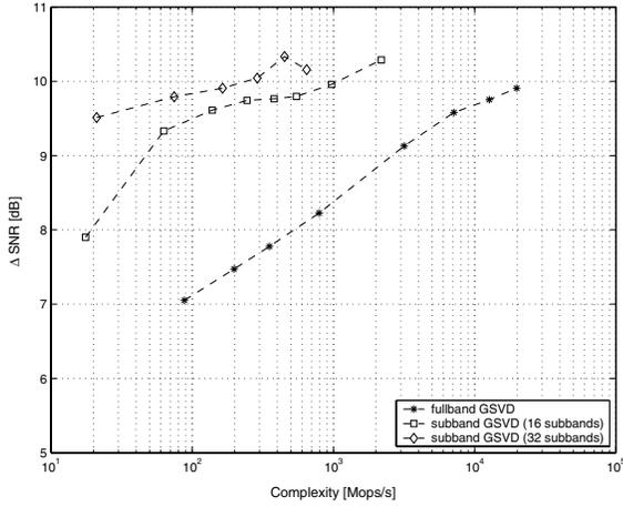
Figure 2: Improvement in SNR of fullband and subband GSVD as a function of complexity (Mops/s) for  $M = 4$ ,  $d_f = d_g = 1$ .
