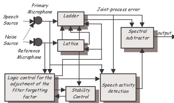
Figure 1. General framework of the proposed methodology: A Lattice-Ladder Filter is combined with a Spectral Subtractor.
