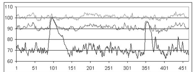
**Figure 7.** Instantaneous energy of the Noisy Speech Trace from Figure 4 (upper trace), of the Joint Process Estimation Error from Figure 5 (middle trace), and of the Speech Trace after Spectral Subtraction from Figure 6 (lower trace).
