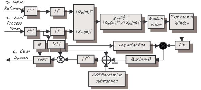
Figure 3: Specific Spectral Subtraction method being proposed
