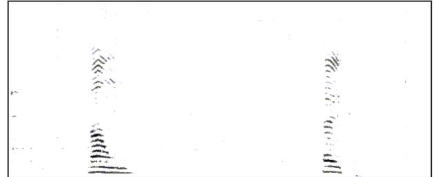
**Figure 6.** Power Spectrum of the Speech Trace after Spectral Subtraction
