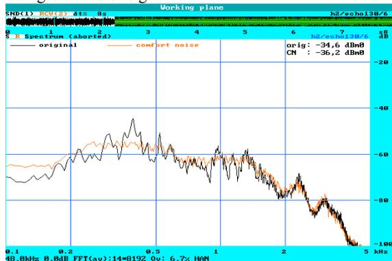
Fig. 5: Spectral difference between transmitted background noise signal before (black) and during far end speech (red/gray)
