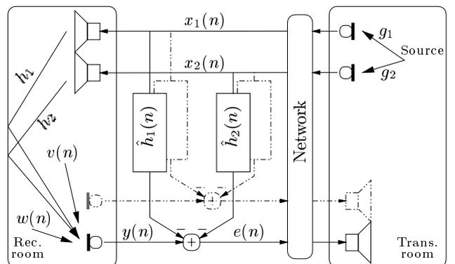
Figure 1: Block diagram of a generic two-channel acoustic echo canceler.
