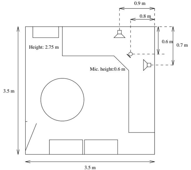
Figure 3: Layout of the office and acoustic setup.
