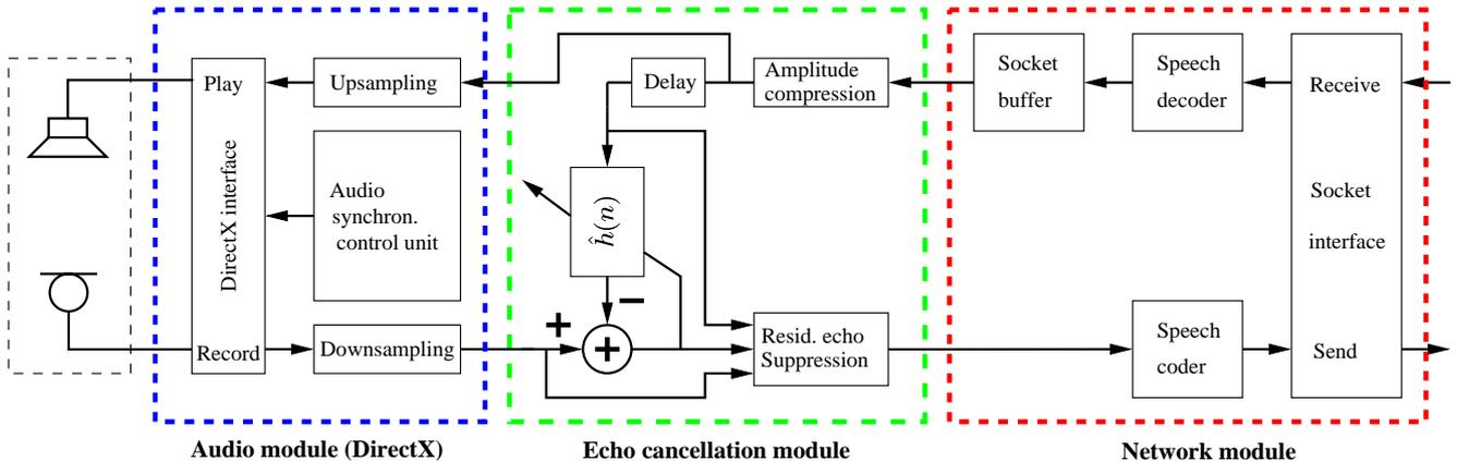
Figure 2: System block diagram for the single-channel case.
