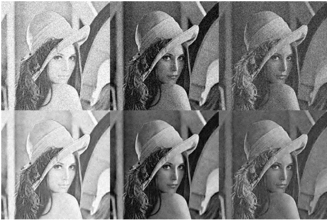
Figure 1: Noisy RGB image components (upper row) and filtered image component (bottom row). Standard deviation of noise in each of 3 image component was 20 with the signal range 0-255. Filtering was performed by filter of Eq. (15) with \lambda_{r_1, r_2, \sigma} = 1 .
