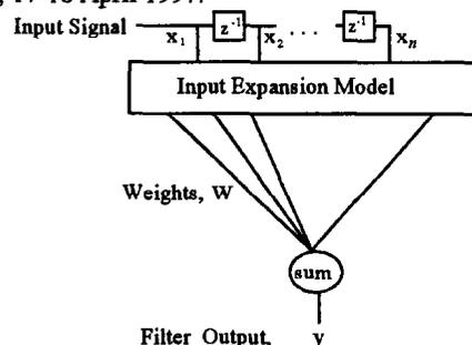
Figure 1: General structure of the proposed ANN Based Adaptive non-linear Filter
